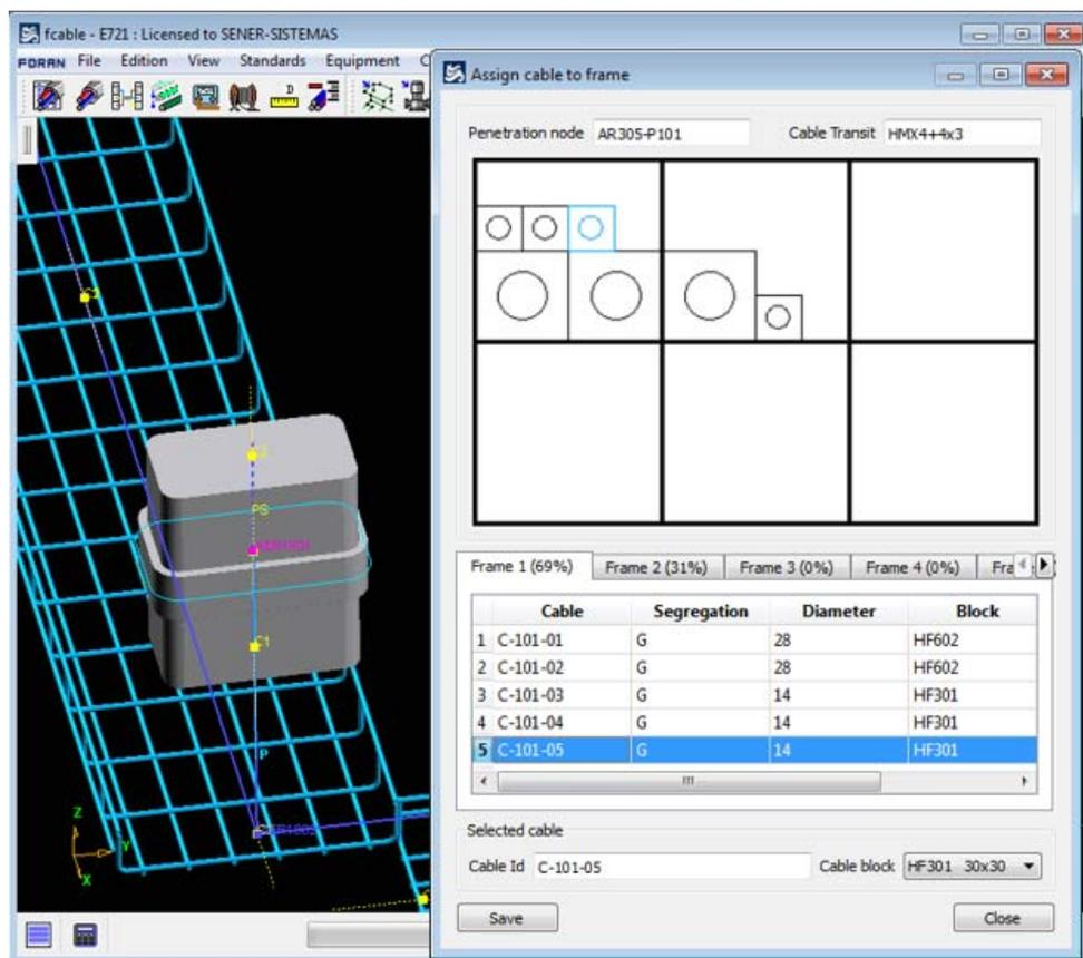
IMAGE: FORAN Cable Arrangement
